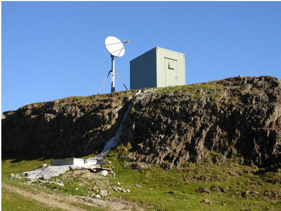
Figure 2. A photograph of the NZNSN station PUZ showing the VSAT dish and equipment hut on top of the rock outcrop. The sensor vault is located in the foreground on the left hand side of the photograph.
