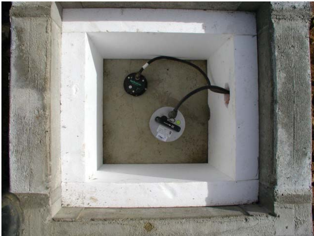
Figure 3. A view of the NZNSN vault at WHZ with a Guralp CMG-3ESP broadband seismometer and Kinematics Episensor installed.
