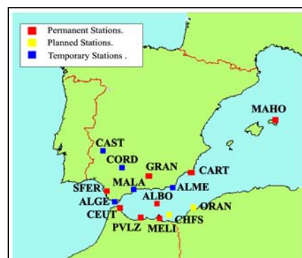
Fig. 2: ROA Permanent (red) and Temporary (blue) GPS nets.
