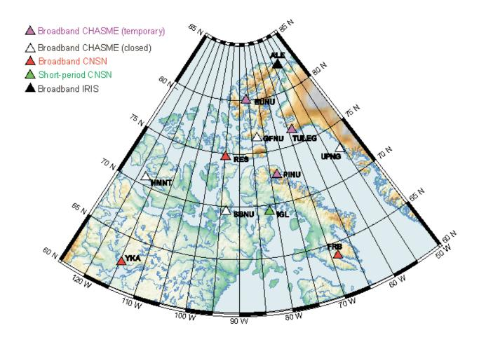
Deployed during the summer of 2000. All but three stations have now been closed: TULEG (Guralp CMG-40T), Pond Inlet (CMG-3), and Eureka (CMG-3). All use Nanometrics Inc. (NMX) Orion data loggers; removable disks exchanged ~ monthly.
